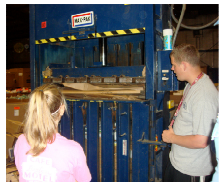
A volunteer uses one of the vertical balers at Pro Kansas Recycling.
